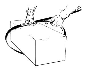
b. OPEN-FLANGE SEAL: Pass the lead end of strap around the package and up beneath top strap. Snap seal(s) over both layers, allowing two (2) inches of lower strap to extend beyond seal(s).
