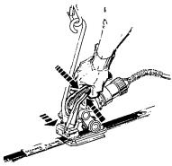
3. While standing to one side of the strap line, rotate the air valve collar, as shown, to tension the strap. Be careful not to lift up on the motor. Instead, press down to assist the gripper wheel action.
