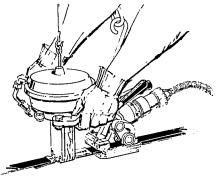
Rotate the air valve collar, as shown, to release the air pressure before cutting the strap.
