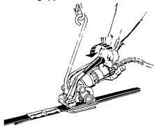
Crimp (or notch) the seal(s) while the strapping is under tension. An air powered sealer, as shown, or a manually operated sealer can be used.
