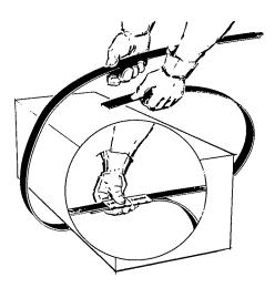
c. Hold seal(s) in place by bending down lower strap. Pull out slack strap and slightly bend the upper strap to maintain position of seal(s).
