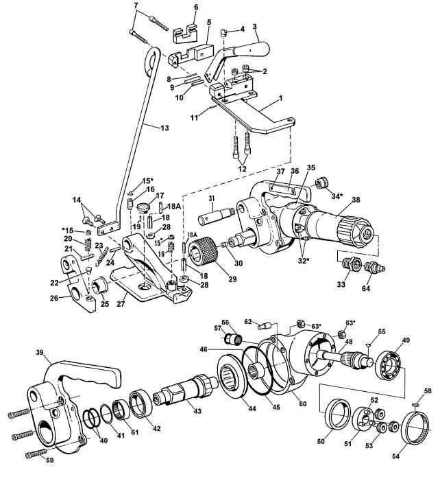
\* Apply one drop of Loctite #242 (P-422795) sealant to cleaned parts. Allow 12 hours to set if possible. Do not apply to small screws or close to moving parts as the liquid spreads easily.
