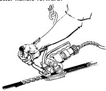
7. To remove the tool raise the motor and twist the front end of the tool away from the tensioned strap.
