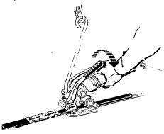
6. Strapping is then cut off by moving the cutter handle forward.
