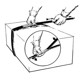
2. Grasp the FN Tensioner with your right hand and squeeze the handles together to raise the feedwheel and the wear plate. Insert the top strap between the feedwheel and the wear plate and insert the lower strap between the wear plate and the base. Both straps must be fully seated against the inner strap slot. Release the handles.
