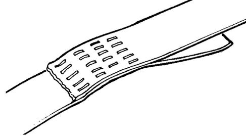
The welded area should extend the full length and width of the gripper impression.
