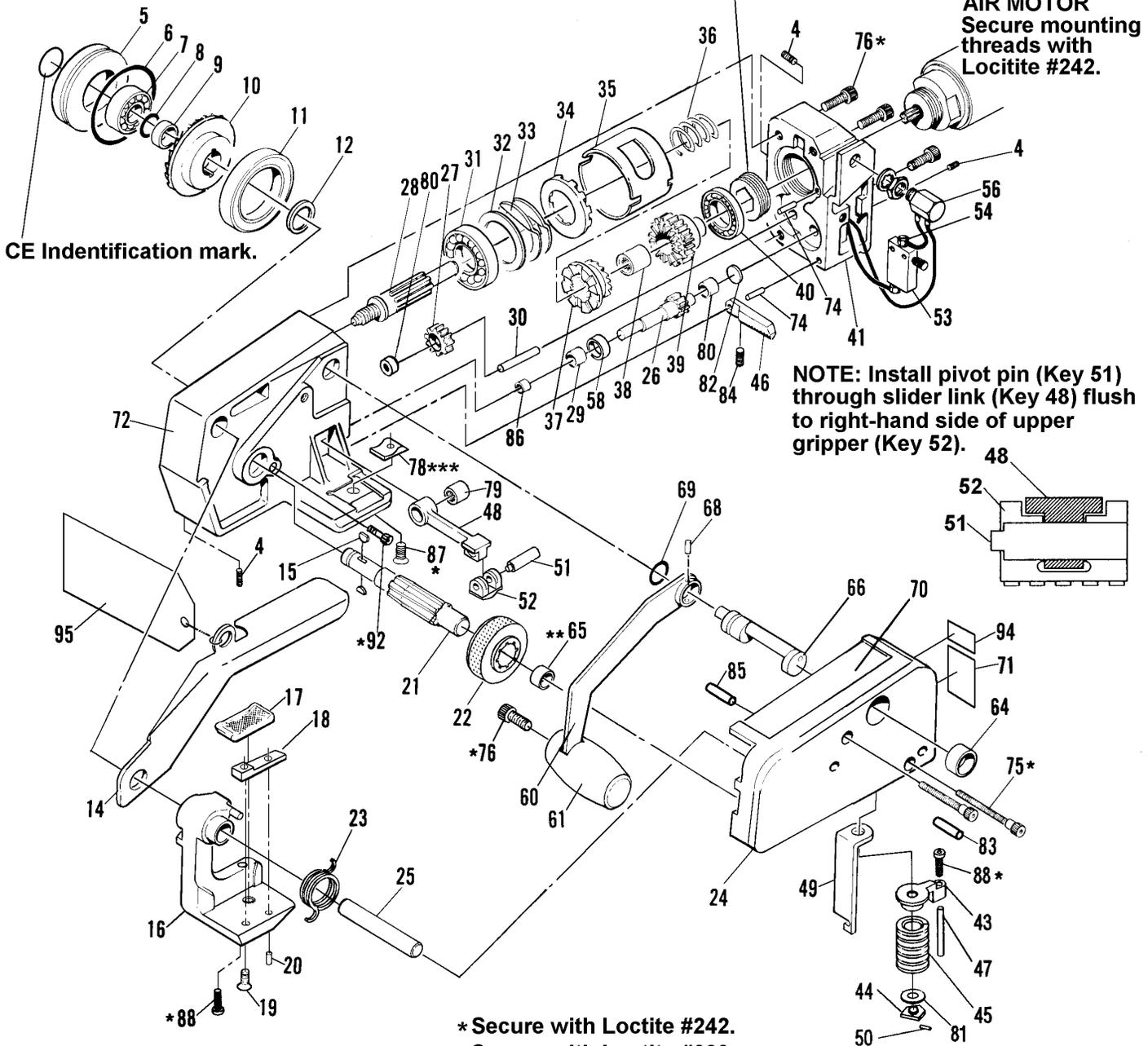
**NOTE:** Install pivot pin (Key 51) through slider link (Key 48) flush to right-hand side of upper gripper (Key 52).
