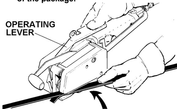
2. Recheck the strap alignment at the rear of the tool and realign if necessary. Release the operating lever and, while standing to one side of the strap line, squeeze the motor control lever to tension the strap.
