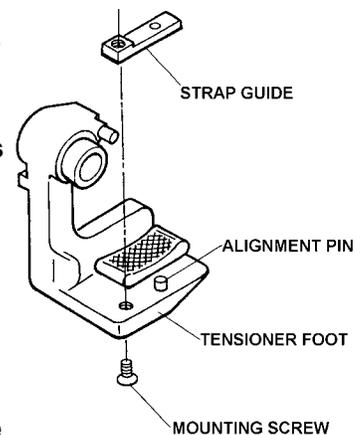
Replace the new strap guide in the same manner in which the old guide was removed.
