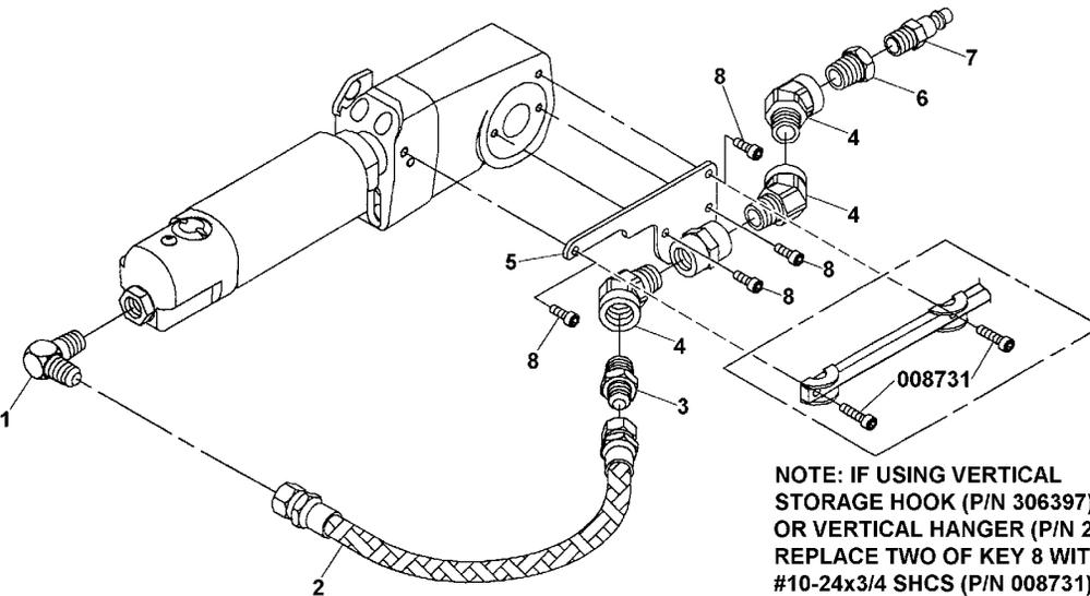
**NOTE:** IF USING VERTICAL STORAGE HOOK (P/N 306397) OR VERTICAL HANGER (P/N 274164) REPLACE TWO OF KEY 8 WITH TWO #10-24x3/4 SHCS (P/N 008731).
