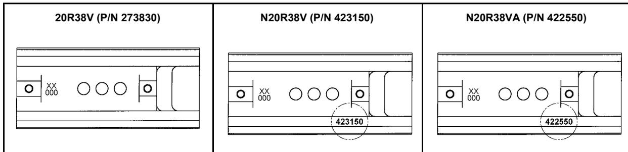
**NOTE:** Air motor 20R38V is an older style air motor used on VXL/VXM tools. Air motor 20R38V can be identified by the absence of a part number engraved or stamped on the underside of the motor housing.
