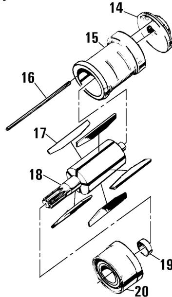
12. Look for areas of wear on the face of the end plates, the pinion teeth on the rotor and the edges of the vanes. The vanes must be kept clean to float freely in the rotor. **Note:** If the vanes and/or the idler assemblies have to be replaced, they must soak in air line oil overnight before assembling them into tool.
