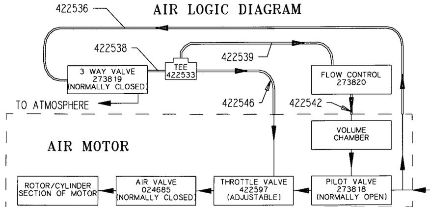
4. The motor lever and weld handle are released and the tool returns to the "at rest" configuration, with air being routed through the pilot valve, throttle valve and stopping at the air valve.
