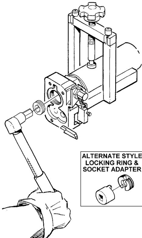
20. Continue to reinstall the O-ring, valve housing assembly, drive gear, bearing and lower air motor cover.
