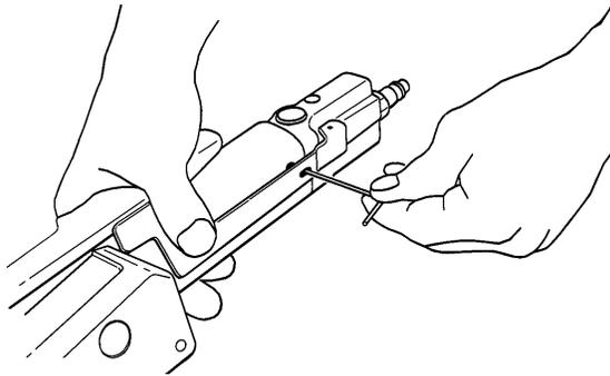
**NOTE:** Operating air pressure must be set between 85 and 90 psi (5.7-6.2 Bar). With accurately controlled air pressure the tension will be uniform on all straps, provided the operator allows the air motor to stall.
