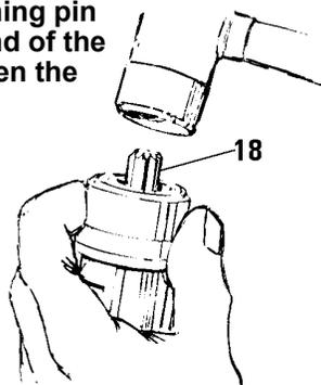
11. Disassemble the rotor by sliding off the front end plate (20), and any ball bearing(s) and spacers. Then slide the back end plate (14) and the rotor assembly (18), with the vanes (17), out of the cylinder.
