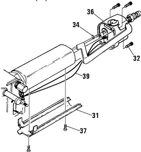
2. Remove the O-ring (34) from the end of the air motor housing. Set it to the side for reuse.
