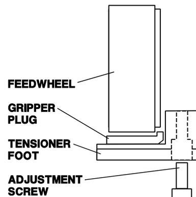
Turn the adjustment screw clockwise for greater clearance and counter-clockwise for less clearance. Turn the adjustment screw only in 1/8 turn increments. After each 1/8 turn, repeat the adjustment testing as described in step 2.
