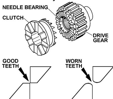
4. With a moderate amount of grease added, a new clutch can be installed on the spline of the Spiroid worm (28) and a new drive gear assembly (39A) can be installed into the motor mount.
