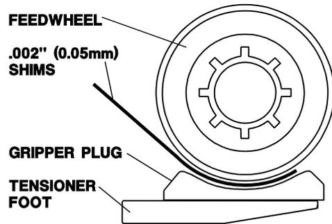
2. Release the tensioner foot to pinch the shims between the feedwheel and the gripper plug. Holding the shims with one hand, jog the air motor on and off to rotate the feedwheel at least one full revolution. If properly adjusted the tool should lightly tug at the shims while rotating. Clearance between the feedwheel and gripper plug at this point should fall between .002"-.004" (.05-.10mm).
