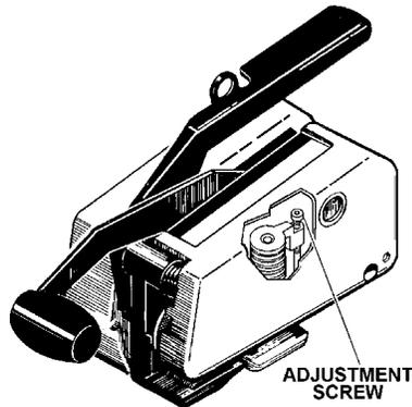
**NOTE:** Do not over tighten cutter mechanism as lower strap damage or poor strap cut-off will occur.
