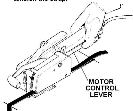
3. When the motor stalls, indicating completion of tension, continue to hold the motor lever fully closed against the motor housing and pull back the weld handle with your left hand. The handle should be pulled quickly all the way back without hesitation. When the weld lever is pulled back it traps the motor lever in the ON position.
