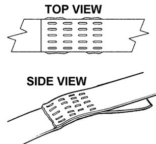
If the joint still does not appear as shown, then inspect the tool for worn and/or damaged parts. Replace tool parts as needed. **NEVER HANDLE OR SHIP ANY LOAD WITH IMPROPERLY FORMED JOINTS.** Misformed joints may not secure the load and could cause serious injury.
